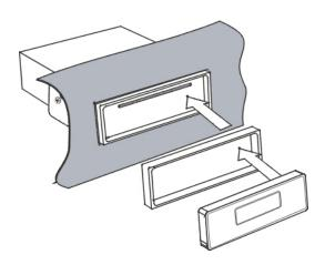
Once the CD player is secured, fit the trim ring over outside edge of the radio until it snaps into place. Insert the face plate with the right side first. Angle in the right side slightly then gently push the left side of face plate until it snaps completely in place.
